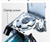
Blade cover can be opened just by loosening clamp screw.
