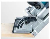
Angle adjustable fence can be locked in any position between 0° and 90° with positive stops at 0°, 45° and 90°.
