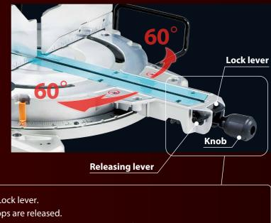
Once Releasing lever is pushed down:
